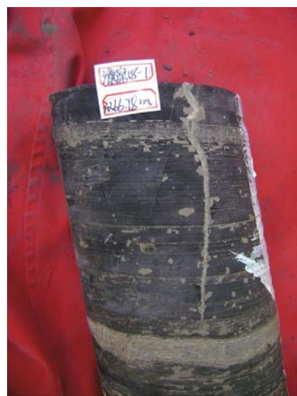
图4 柳屯洼陷 PS18-1 井裂缝在不同岩性中的发育 Fig. 4 Development of fractures in different lithologies in the well PS18-1 of the Liutun sag
